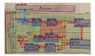
Fig. 3: *Step 1*: Candidate shapes and edges have been classified and localized through bounding boxes, in addition edges have predicted arrow head ( $\triangleright$ ) and tail ( $\circ$ ) keypoints.
