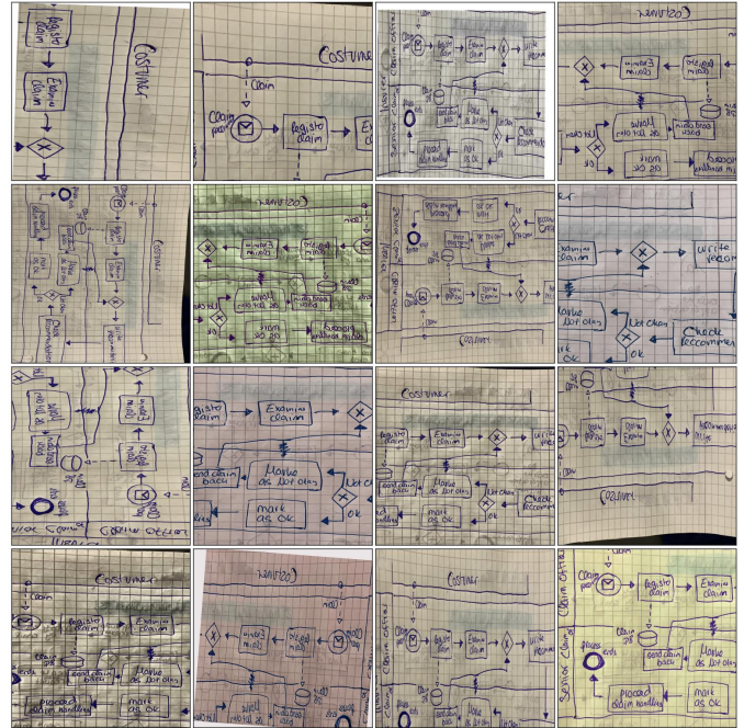
Fig. 14. Image Augmentation Example: Our augmentation pipeline produces different variations of the same input image
